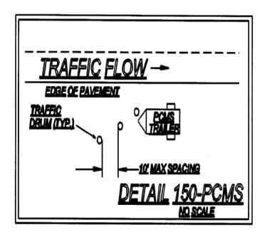
When not in use the PCMS shall be removed from the roadway unless protected by positive barrier protection. If the PCMS is protected by positive barrier protection the sign panel shall be turned away from traffic when not in use.
