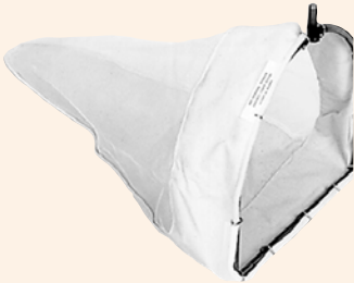
A D-frame fine-mesh dip net for collecting macroinvertebrates.
